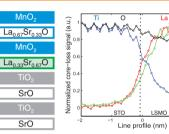
Compositional interface engineering prevents reconstruction at the  $La_{0.67}Sr_{0.33}MnO_3/SrTiO_3$  (LSMO/STO) interface caused by polar discontinuities in perovskite oxide epitaxial heterostructures. The polar discontinuity at this interface can be removed by the insertion of a single  $La_{0.33}Sr_{0.67}O$  layer, resulting in improved interface magnetization and electrical conductivity.
