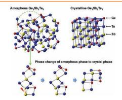
In the rapid phase change material  $Ge_2Sb_2Te_5$ , the Ge-Te core network stabilizes the amorphous phase at room temperature. This network is also present in the crystalline phase, thus enabling rapid phase change. The Sb-Te pseudo network, defined by atoms that are somewhat further apart than the covalent Sb-Te distance, is responsible for triggering critical nucleation.
