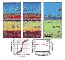
Through selection of an appropriate adhesion layer for platinum on silicon, an ability to process complex oxide thin films devoid of chemical gradients is demonstrated. The chemically homogeneous films display significantly enhanced electronic and dielectric responses across two separate material systems, PZT and BaTiO<sub>3</sub>, with nearly 35% increases in remanent polarization and 300% increases in permittivity observed, respectively.
