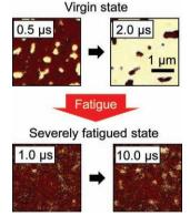
A time-dependent domain wall pinning process is found using modified-piezoresponse force microscopy studies to be the microscopic origin of polarization fatigue. Nanoscale domain switching dynamics are visualized directly for different fatigue stages in epitaxial ferroelectric thin films. The evolution of domain wall pinning is directly observed from the suppression of sideways domain growth to the blockage of forward domain growth during fatigue.
