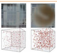
A full 3D reconstruction of pores in transparent polycrystalline alumina is performed, demonstrating that pores smaller than ≈50 nm have a drastically smaller effect on the degree of transparency than commonly presumed. Furthermore, how to quantitatively incorporate the pore characteristics into the conventional optical transmittance model by deterministically modifying its input parameters is shown.
